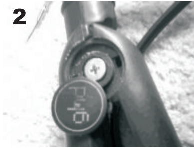
2. Remove both sides, to reveal the screw head as above
