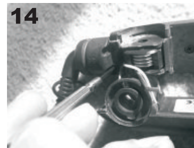
14. Screw the cover plate back over the pin and connector.
