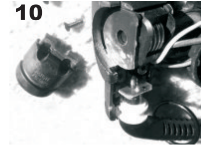
10. This will now reveal the cable pin and connector.
