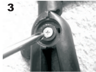
3. You will need 2 phillips head screwdrivers to remove the hinge pin
