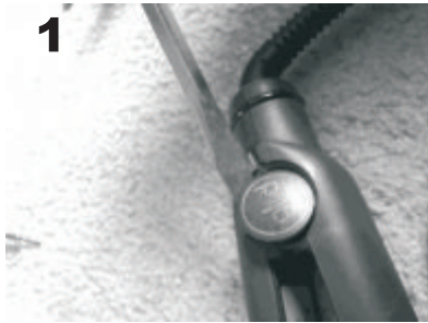
1. Remove the hinge covers with a flat head screw driver
