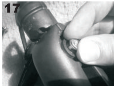
17. Then push the other hinge screw back in place.
