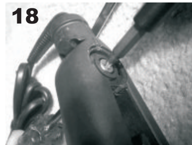
18. Again using 2 screwdrivers, tighten the hinge pin until secure.
