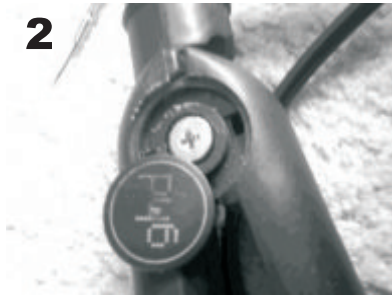
2. Remove both sides, to reveal the screw head as above
