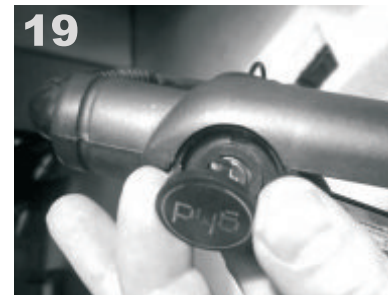
19. Replace the 2 hinge covers back to cover the screws.
